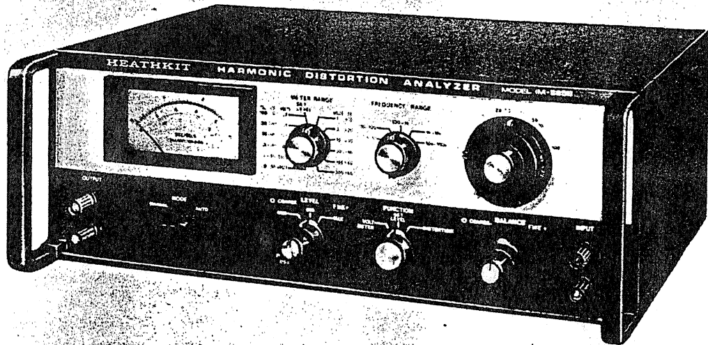
FIGURE 3-30. The Heathkit® IM-5258 Harmonic Distortion Analyzer, which is tuneable over a wide frequency range. Courtesy of Heath Company.
