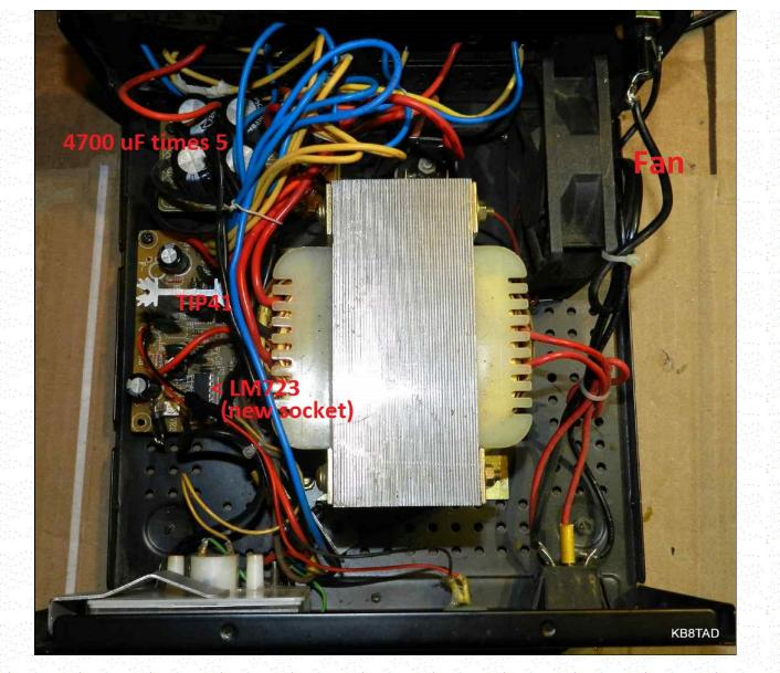
I puzzled over the thermal switch but that part was working properly. It only sees the current from the TIP41 transistor fed to the bases of the pass transistors. On powering the unit up slowly, I found it working. I cleaned the voltage adjustment variable resistor (VR-2) and checked its setting to verify 13.8 volts output. A load test verified a fully functional power supply. Power had returned to the Pyramid.
