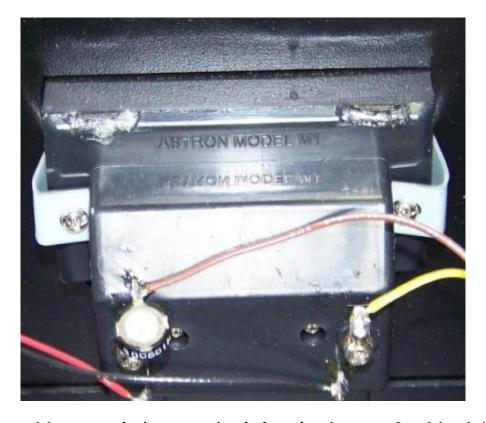
Once I removed the meter *and prior to removing the lower housing screws* I used dental picks and a razor blade to remove the glue and separate the housing lip. Prying gently outward until I made certain the housing would come apart once I removed the 2 lower screws holding the meter front to the housing.
