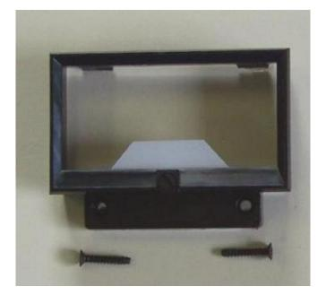
2 small screws hold the meter scale in place. I removed the scale. Behind it I found 2 glass lamps (resembling a small glass fuse) mounted on a circuit board.
