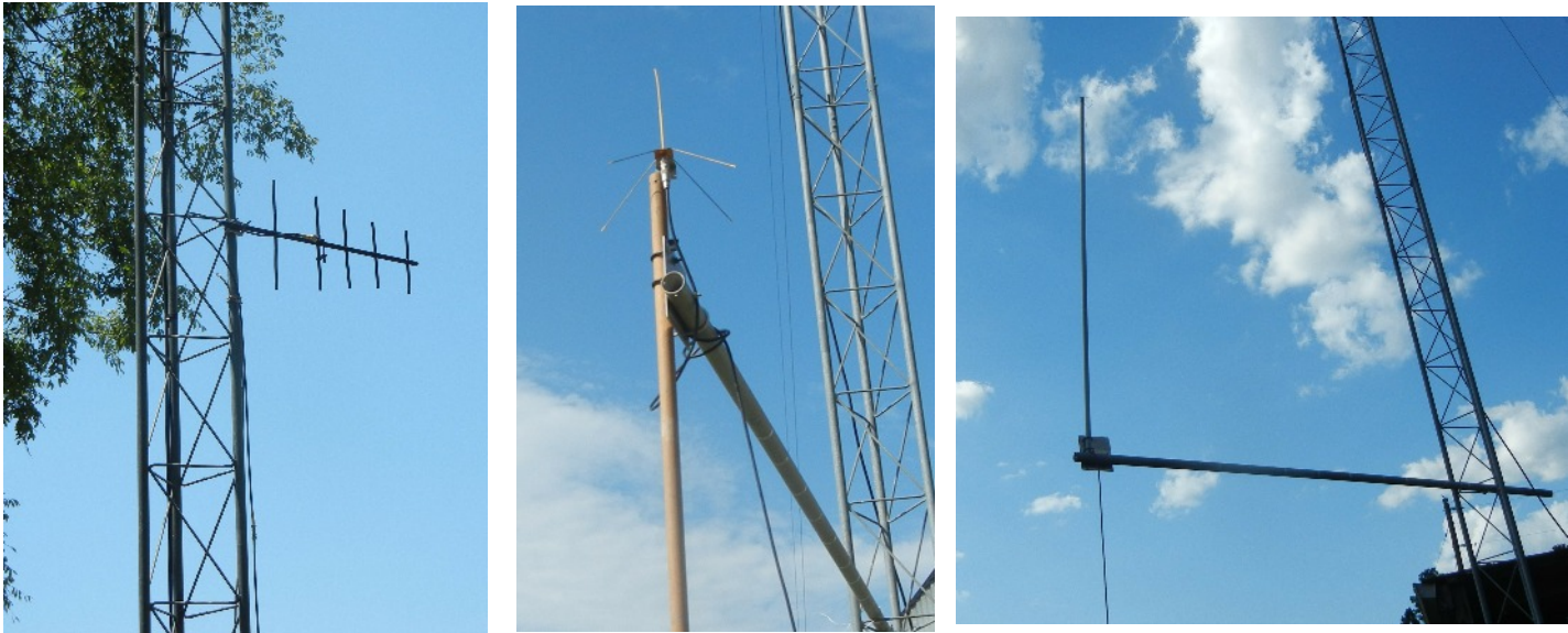
Figure 10. Left to right; 5 element yagi receiving antenna, \lambda/4 reference antenna and AUT.
