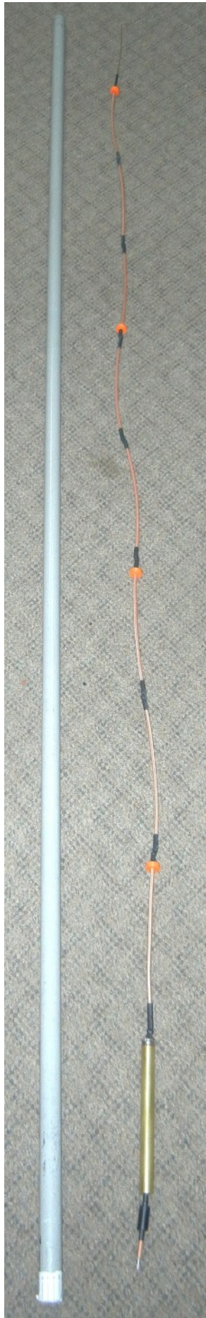
Figure 8. Assembled antenna ready to mount in radome and install type-N test connector.
