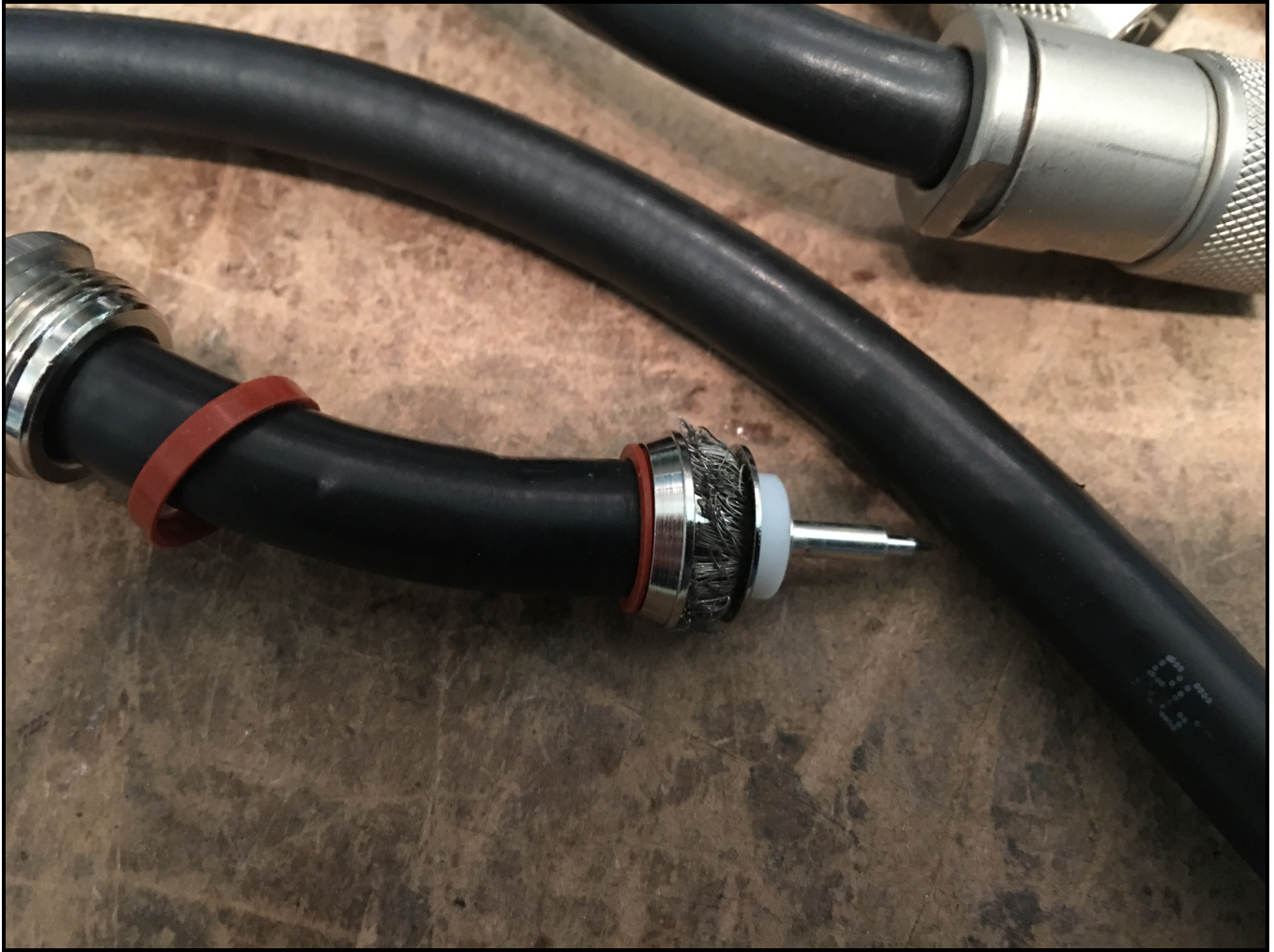
ORIGINAL HARNESS CONNECTOR DISASSEMBLED
