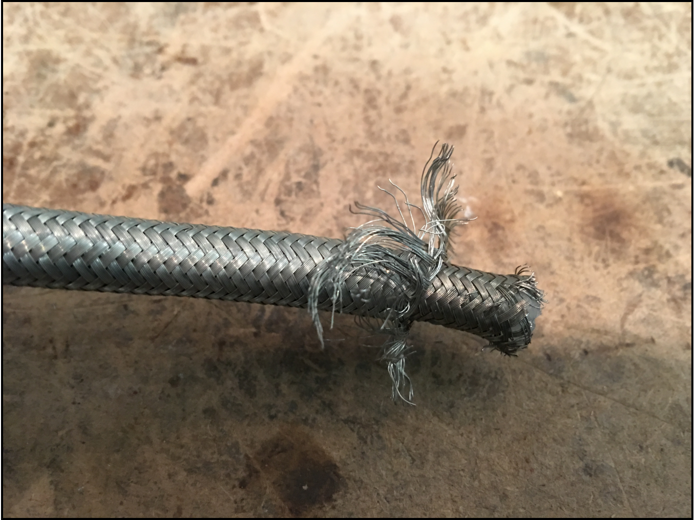
RG-214 "TYPE" CABLE - DOUBLE TINNED-COPPER BRAID
