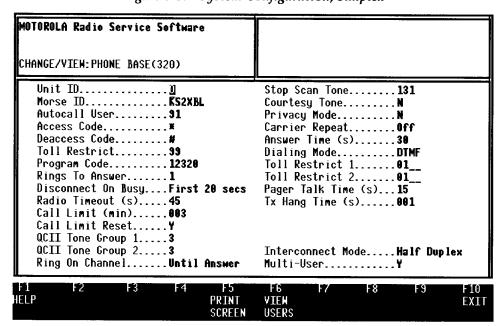
Figure 6-4. System Configuration, Duplex
