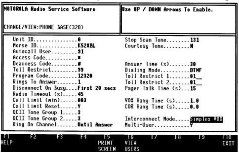
Figure 6-3. System Configuration, Simplex
