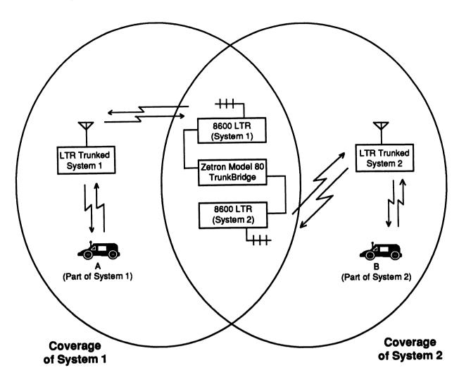
This mode of operation is the reason the Model 80 is called the "TrunkBridge." When the TrunkBridge is connected as shown above, selected users from two LTR trunked systems are allowed to communicate with each other. In full TrunkBridge operation, the TrunkBridge is connected to two 8600 series LTR radios. Each radio belongs to a different system. The same system and group slots are programmed on both radios.
