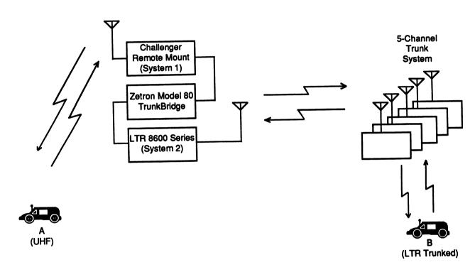
The capability of allowing a conventional radio system and a trunked radio system to communicate with each other is a powerful feature of the Model 80 TrunkBridge. In this configuration, a VHF or UHF Challenger remote mount radio is connected to the system 1 input of the TrunkBridge, and an 8600 series LTR radio is connected to the system 2 input of the TrunkBridge. As with the other two TrunkBridge configurations, both radios are placed in scan when the system is initially placed in service.
