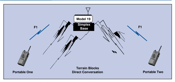
Step One: Portable one transmits; the Model 19 records audio from portable one received by the simplex base station.
