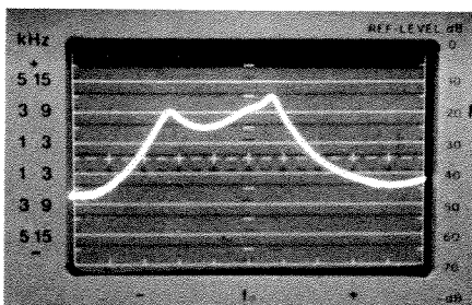
CRT Photo 1 shows a badly aligned RF filter that is located in the front end of a receiver.
