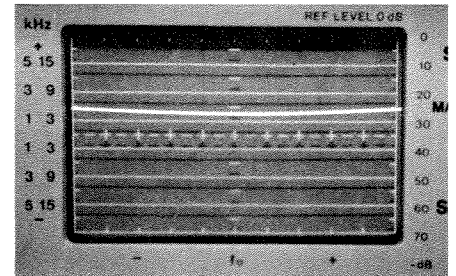
CRT Photo 1 shows 27 dB of rejection for reverse power in the first section of a two section isolator.
