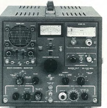
CE-7. Ideal for applications with a limited number of operating frequencies. 23 crystal-controlled channels can be selected between 20 MHz and 1150 MHz. The instrument also generates up to ten different crystal-controlled IF signals between 250 kHz and 20 MHz.
