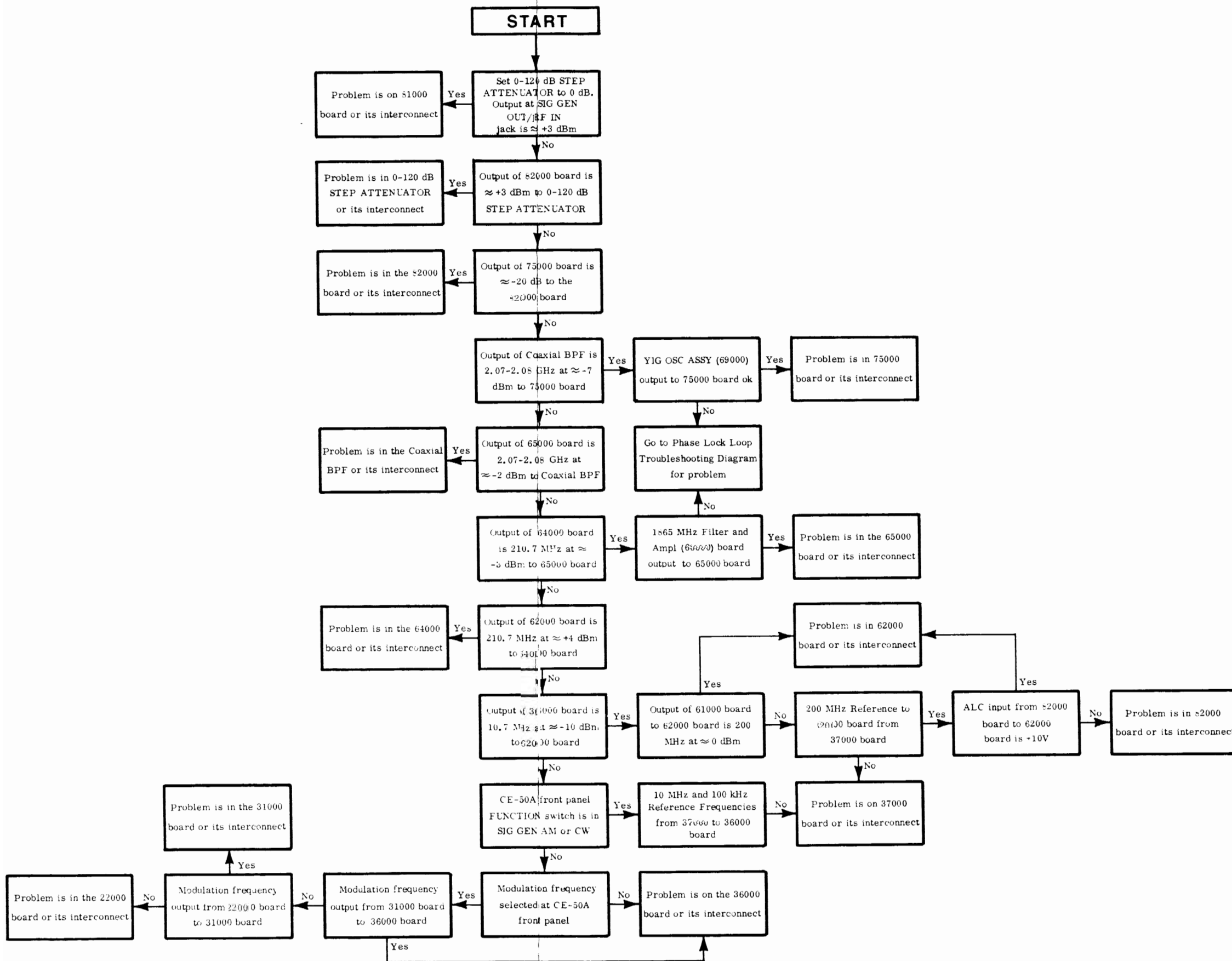
Figure 5-7. Signal Generator Troubleshooting Diagram
