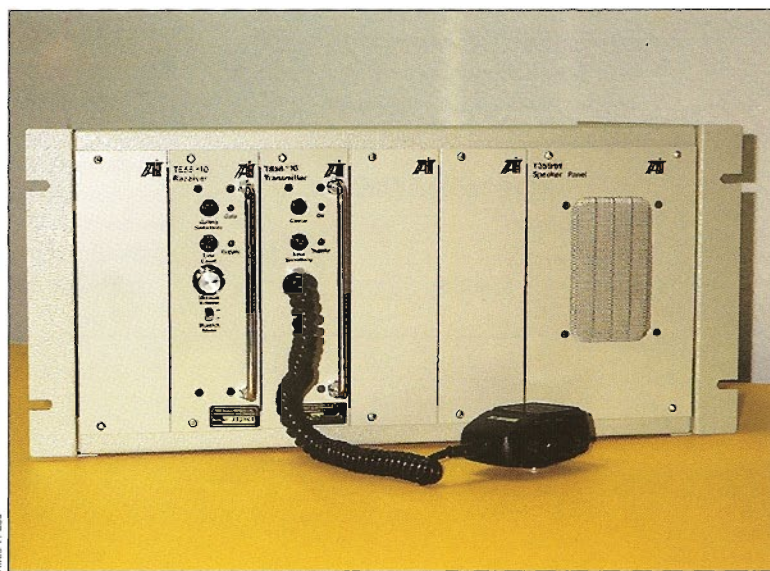
The Model T855-10 receiver and T856-10 transmitter modules from Tait Electronics, Ltd.
