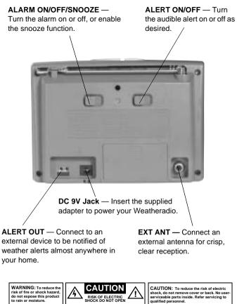
The lightning symbol is intended to alert you to the presence of uninsulated dangerous voltage within this product's enclosure that might be of sufficient magnitude to constitute a risk of electric shock. Do not open the product's case. The exclamation symbol is intended to inform you that important operating and maintenance instructions are included in the literature accompanying this product.
