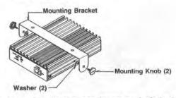
Note: The mounting knobs are large and slotted so you can easily tighten them with either your fingers or a large flat-blade screwdriver. Do not over-tighten.
