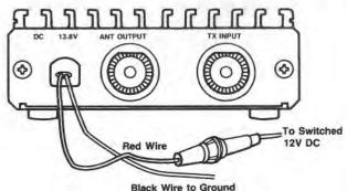
Connect your transceiver's antenna RF cable to the TX INPUT connector on the back of the amplifier.
