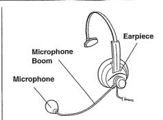
Your RadioShack Single Ear Mono Headset with VOX (Voice Activation) allows handsfree operation of your mobile or handheld communications transceiver. You can use this headset with many of the RadioShack handheld amateur radio, business band, FRS (Family Radio Service), and citizen's band transceivers that have external microphone and speaker jacks.
