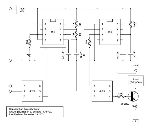
Note 2: The schematic above shows a 220 uF timing cap in the monostable, which was used in a different system where a longer run time was desired (approximately 9 minutes)
