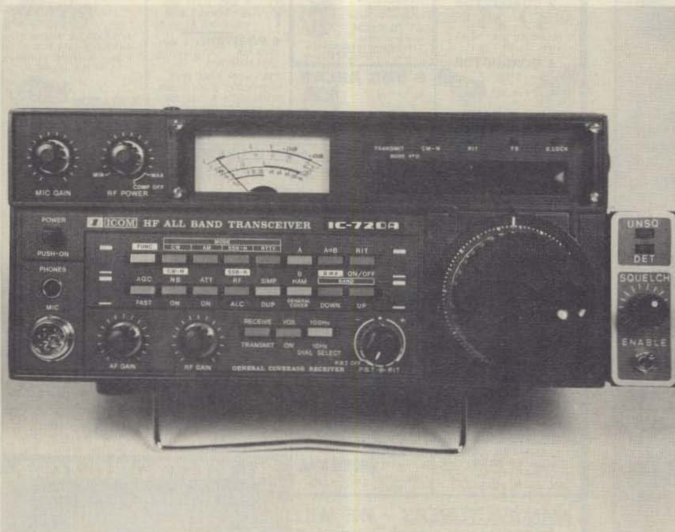
Photo A. Squelch unit is attached to the right side of the HF SSB transceiver. Rectangular LEDs above the control knob indicate circuit status. (Photo by KA9FJS)
