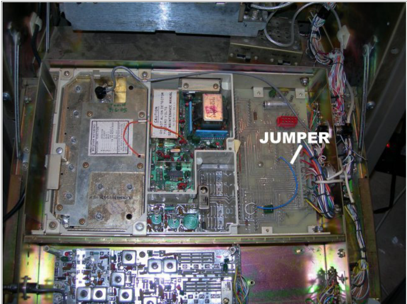
Illustration 4: CTCSS Jumper Installation on System Board
