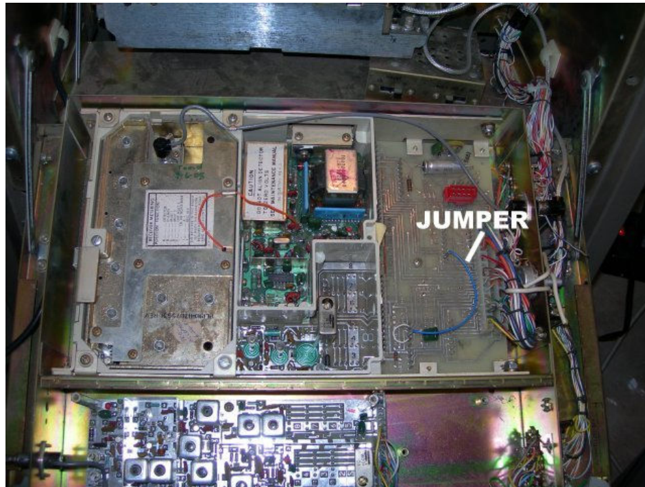
Figure 4 Jumper Placement for CTCSS Encoding
