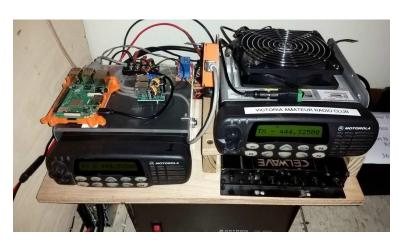
acquaintance gave me a pair of radios to build a repeater and copy of the programming software or CPS. From that point I saw the value of working with the newer synthesized Motorola radios. The repeater we built with the two Motorola CDM-1550
