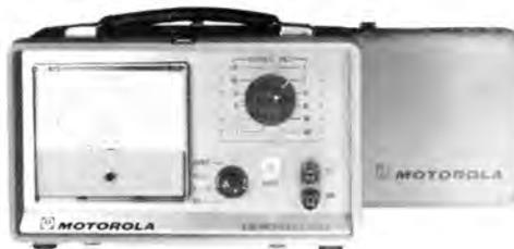
Transistorized AC Voltmeter
