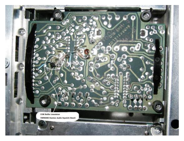
Steps 4-11 convert the station version of the audio/squelch board (TRN-6006A) to be more useful for ham controller use. See reference 5 for detailed instructions. The meat of the conversion is replicated here.
