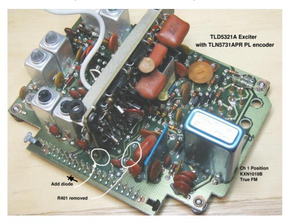
2). There are two options of modification to allow proper keying of the exciter if
