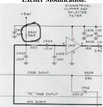
1.) See reference 1. Remove R401 to increase tx audio input impedance and to remove the dc bias from the mic audio line.. This is most likely a 560 ohm resistor. On the board in my base station, this resistor had already been removed.
