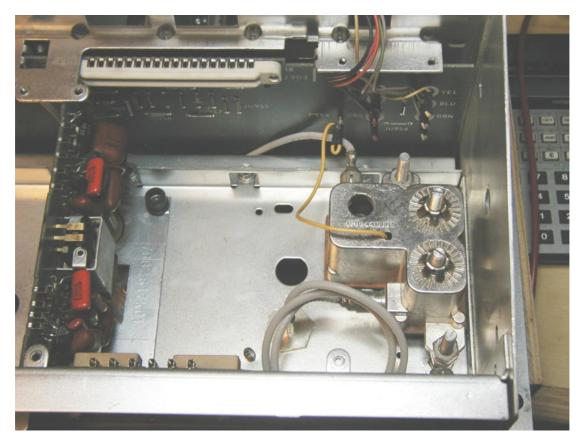
12) Add a 4k7 resistor from J2-10 to ground. This gives a load for the PL detect signal. I found operation with the RLC was intermittent without the pull down. The voltage swing at J2-10 should be 0.3(no PL) to 9.0(PL detected) with the controller plugged in. There is a convenient ground connection down and right of J2-10. Its the heavy trace leaving the J1 power connector.
