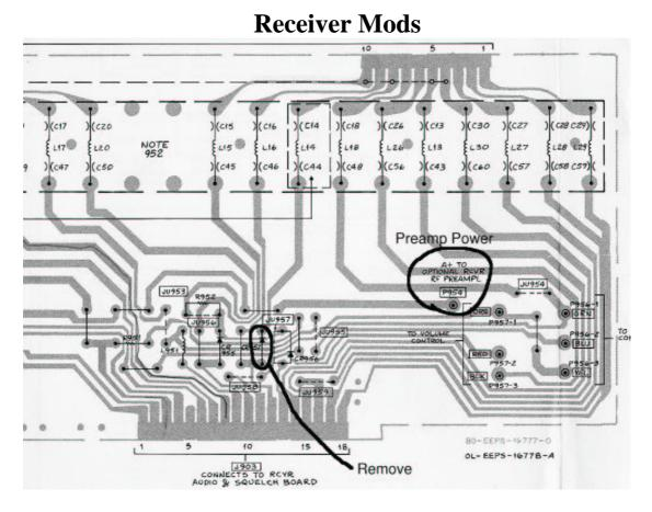
1).Remove CR 957 on receiver interconnect board (the board that lays horizontally between the backplane and receiver board) so that receiver will not be muted when transmitter is keyed. CR 957 is the diode located between JU958 and JU957 on the right hand side of the interconnect board by the audio/squelch board connector. (use the diode for the exciter mod above)
