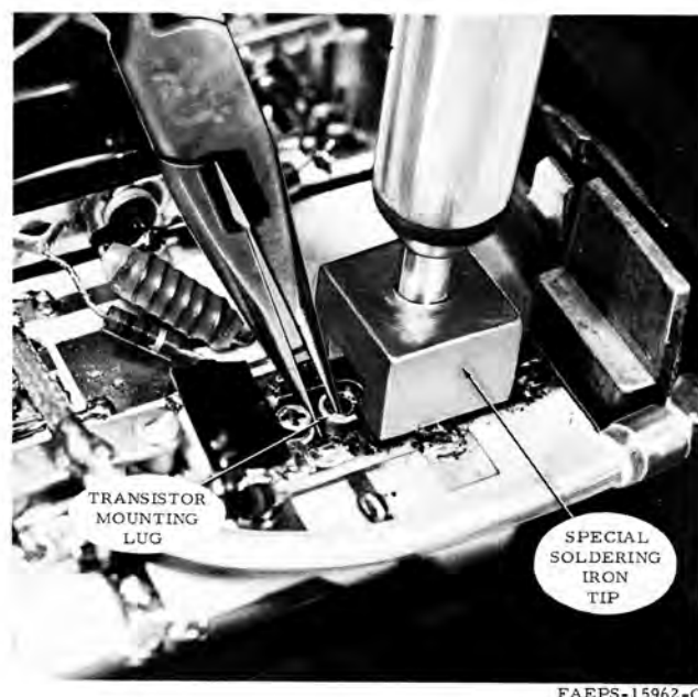
Figure 10. Power Transistor Removal, Using ST-1161 Soldering Iron Tip
