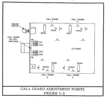
a. Insert the Call Guard card into the card rack with an extender card. Cut the frequency range jumpers for each Call Guard as shown in Table 5-5.
