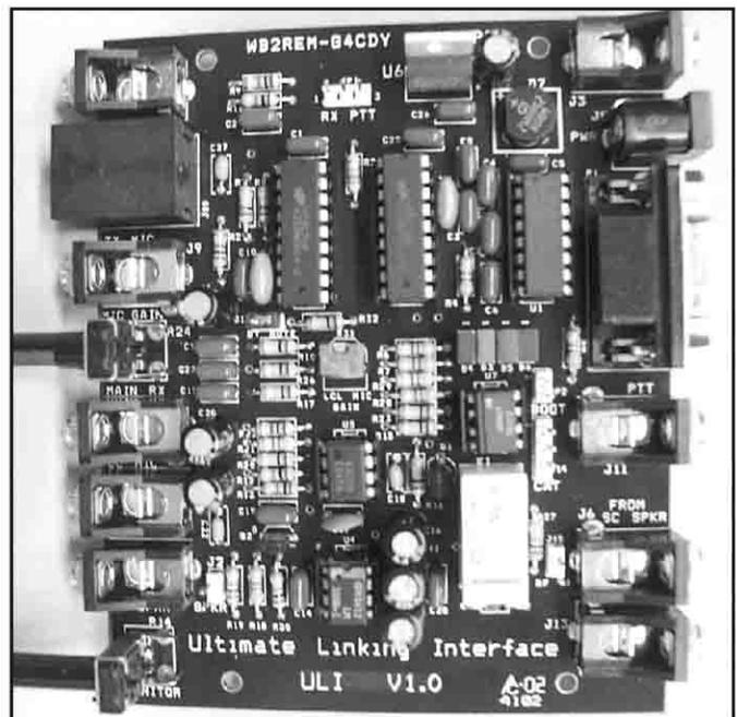
The advanced ULI interface can be used with iLink, EchoLink and eQSO, as well as other Amateur Radio digital modes such as RTTY and PSK31. The ULI offers versatile remote control capability. See [www.ilinkboards.com](http://www.ilinkboards.com).
