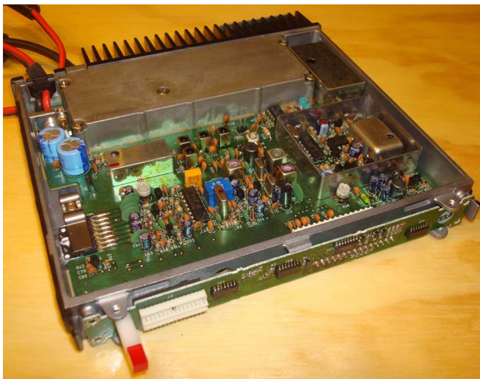
Figure 2. An ICOM UX module with covers removed.
