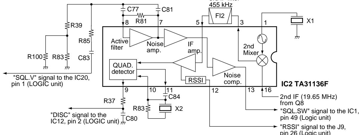
The 455 kHz 2nd IF signal is applied to a ceramic band-pass filter (FI2) where unwanted signals are suppressed and then to a limiter amplifier section in system IC (IC5, pin 5).
