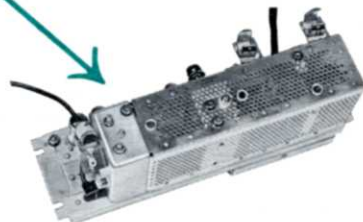
The "Building-Block" transmitter chassis. Interchangeable between mobile and station combinations.
