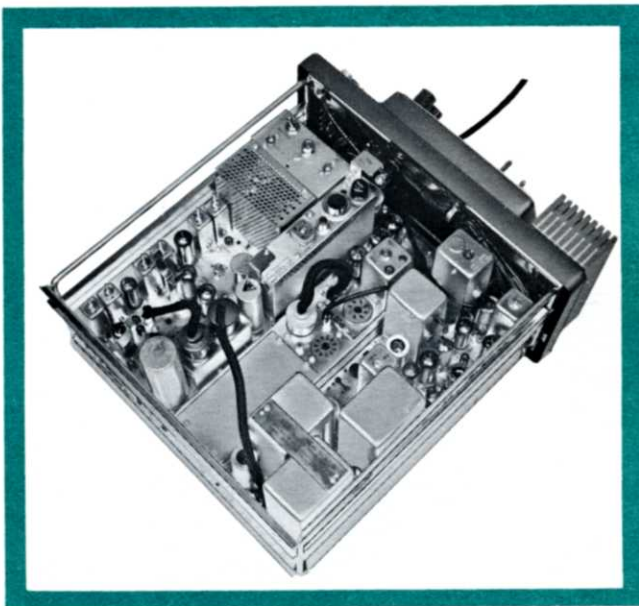
Tone Unit —mounted on option chassis in 14-inch Transistor-Powered Progress Line Mobile.
