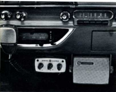
Small control head can be mounted closer to the driver than previously possible.
