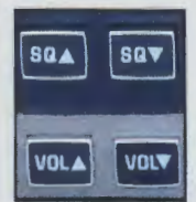
Electronic volume and squelch controls for higher reliability.
