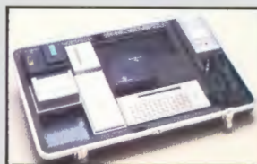
The GE Universal Programmer lets you quickly and easily field-reprogram radio channels, Channel Guard tones, digital Channel Guard codes and Carrier Control Timer intervals.
