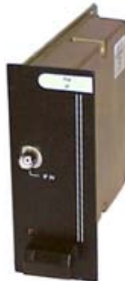
EA101401V1 RX IF Module, P25 21.4 MHz, WB/NB (VHF, UHF)
