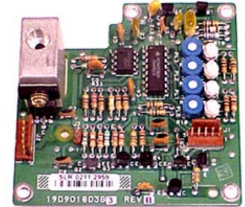
19D901803G3 Power Control Board (Used in 19D901841G3 800Mhz PA)
