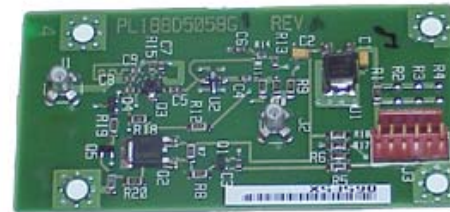
188D5058G1 Buffer Amplifier Board (800 MHz) (Used in 19D901841G3 800 MHz PA)
