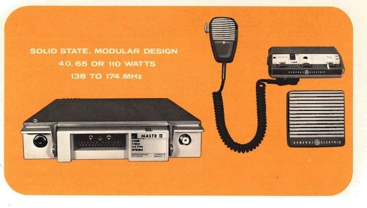
THE MASTR II MOBILE RADIO is a top performance, widely applicable quality radio for today's two-way communication systems. It is the radio with the "built-in future", able to handle system requirement changes expected to occur in the years ahead. Most of its circuitry is composed of plug-in modules which enable field modification or servicing to be quickly and inexpensively performed without unsoldering.
