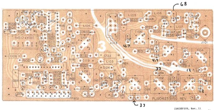
For Ham Radio Frequencies in 52-54 MHz range make the following capacitor changes of the Exec II LoBand 42-50 MHz exiter making it easier to tune.
