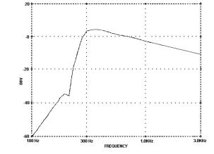
Figure 1 - Channel Guard Tone Reject (+1, -3 dBV)
