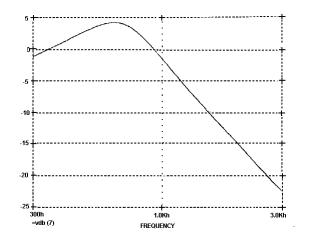
Figure 4 - Battery Alarm/Morse Code Band-Pass Filter
