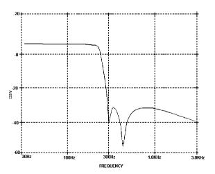
Figure 3 - Channel Guard Encode/Decode Filter
