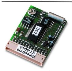
All three popular signaling formats are available in one unit. PC Programmable encoder interfaces with all FM transceivers. Small size makes it perfect for handhelds and mobiles, and low profile connector makes programming and installation a snap. Uses ST-804PM Product Manager software, available for free from our web site, or at a nominal cost from our factory.
