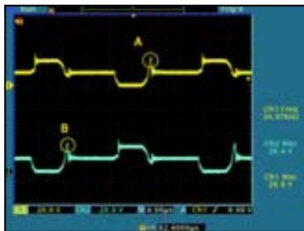
Figure 4—The drain to source voltages of Q5 and Q6 while operating the supply at a load of 300 W. The input voltage was between 10 and 11 V dc. The output voltage was set to 14 V dc. Note points A and B showing the transients generated during MOSFET turn-off.
