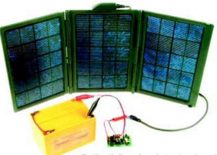
The Micro M+ Charge Controller board, small enough to mount inside your rig, is shown connected to a solar panel and a rechargeable battery.
