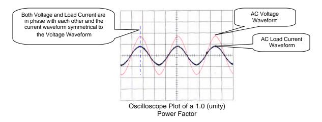
A poor power factor can be the result of either a significant phase difference between the AC Voltage and AC Current measured at the load, or can be due to a high harmonic content or a distorted/discontinuous load current waveform.
