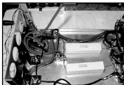
Figure 2 — Internal view showing wiring before switches and 2 Ω resistors are installed.
