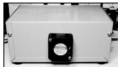
Figure 4 — View of fan mounting arrangement on one side of the aluminum box.
