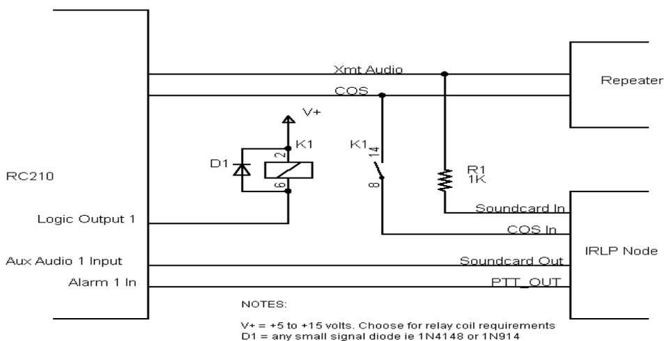
Note that the relay is used to allow remote control of access to/from IRLP (think of it as “link/unlink”). If you want IRLP access full time and don’t need to be able to disconnect it from your system, you may ignore the relay and make a direct connection from the repeater’s COS to the IRLP COS input. Either way, set the IRLP COS selection to Active High or Low depending on your COS signal.
