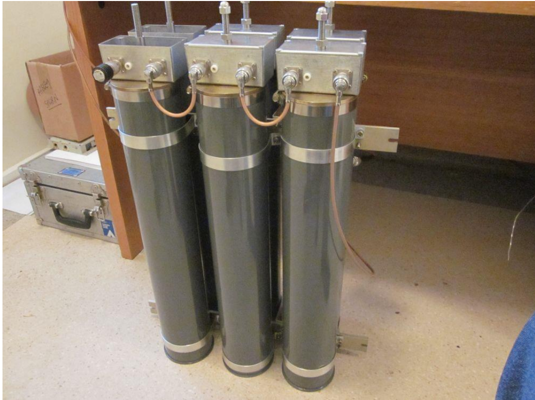
The W1GAN duplexer nearing completion after refurbishment showing 19" rack-mount frame and lugs
