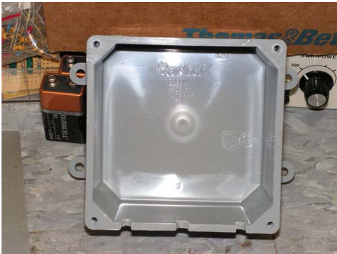
Figure 3 — Notches for the coax were made by drilling holes of an appropriate size near the bottom edge of the box and then using a small file to form the notch. A utility knife was used to clean the remaining debris from the notches.
