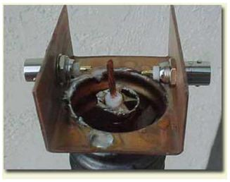
The new design has a box made of medium wall copper bent into a U shaped channel. The BNC connectors are mounted to the walls of the box to add strength. The box is soldered to the top of the Heliax stub. The other major change you will notice is that the coax gimick cap is now a piece of brass hobby tubing soldered into the center of the heliax, this takes the place of the braid that was around the coax in the old design. The center conductor and dielectric is removed from the RG8
