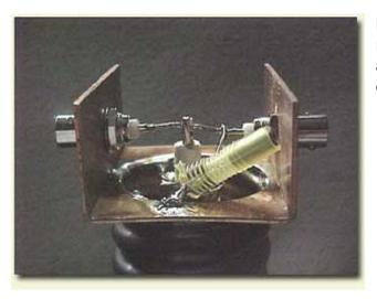
Here is a completed stub with the reactance inductor that has been tuned and ready for service. Very simple and easy to tune.
