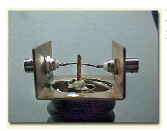
This is how the completed stub looks with the Utah cap and the thru-line conductor. Notice the blob of solder on the plate, this is where the reactance inductor will go.
