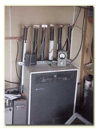
Here is the completed set in service. The whole project took under 10 hours to build and tune however I built one 6 months ago so it was kind of easy. The new design is quieter as I noticed that the old coax braid gimick cap had a tendency to be microphonic, the Utah Cap is much quieter and predictable when it comes to tuning.
