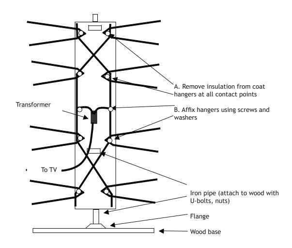
Step 7 Attach wood to pipe with U-bolts.
