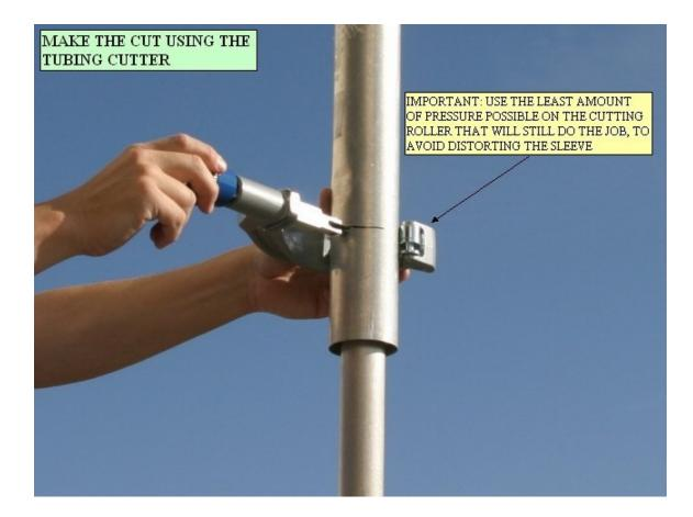
Step 6: After the piece is cut from the sleeve, cut the piece near the lower dimples on both sides of the sleeve and remove the plastic spacer from the inside. If nylon screws hold the spacer in-place instead of dimples, remove them and use the same method (below) to free up the spacer for removal:
