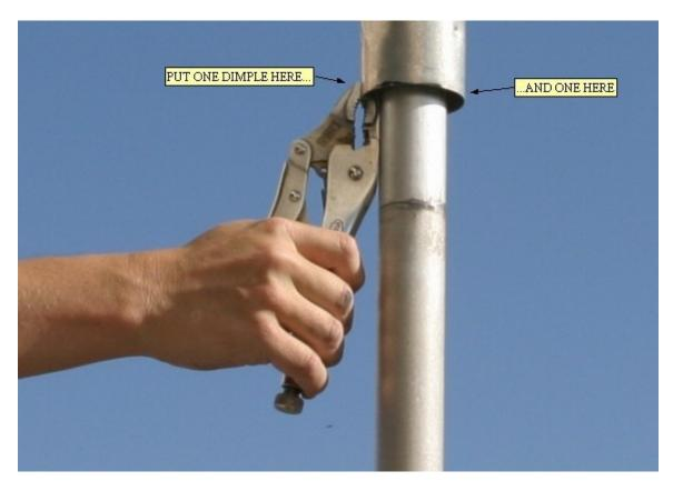
This completes the modification. The antenna may now be swept to confirm that the desired operating frequency is within the acceptable SWR range. A standard tuning ring may be added to lower the antenna's resonant frequency up to about 800 KHz if needed.
