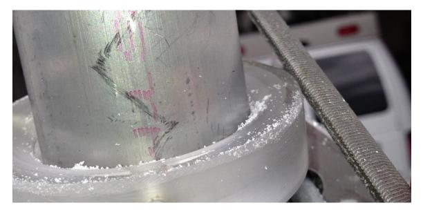
Step 8: Use the custom precision dimpling tool to make two dimples, both as high in the sleeve as possible (about 1.5 inches). Put them on opposite sides of the sleeve. These will prevent the plastic spacer from working its way up too far into the sleeve.
