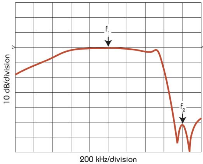
Figure 44. Frequency Response of a 3-Cavity Bandpass Filter in Series with Two Notch Cavities
