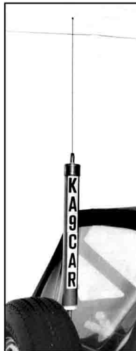
Figure 1—KA9CAR's sleeve dipole mounted on his vehicle.
