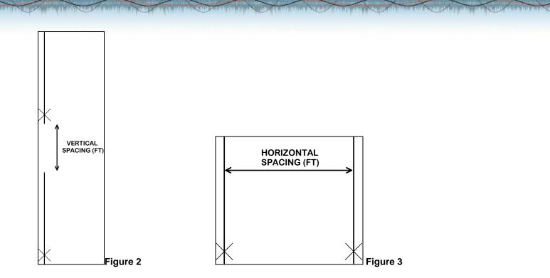
Note that multiple TX antennas can be mounted at the same height, however the worst case spacing between any of them and any receive antennas should adhere to the vertical spacing's listed above.
