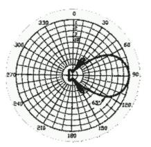
If a reflector is placed next to a dipole all the energy that would have radiated in the direction of the reflector is now reflected back in the direction of the dipole. This makes all the energy appear in only one hemisphere and thus results in a doubling of radiated energy in this direction or 3dB gain.
