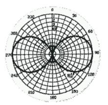
To start with let us take a standard ½-wavelength dipole and "suspend" it in free space (i.e. ignore all possible surroundings e.g. the mounting pole etc. that could affect the antenna). The radiation pattern of this antenna is typically referred to as the "doughnut" as shown in the adjoining figure.
