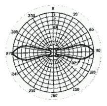
This focusing can be even further intensified such that gains of 6dB (4 times) to 9dB (8 times) can be achieved. The resultant two patterns shown below.
