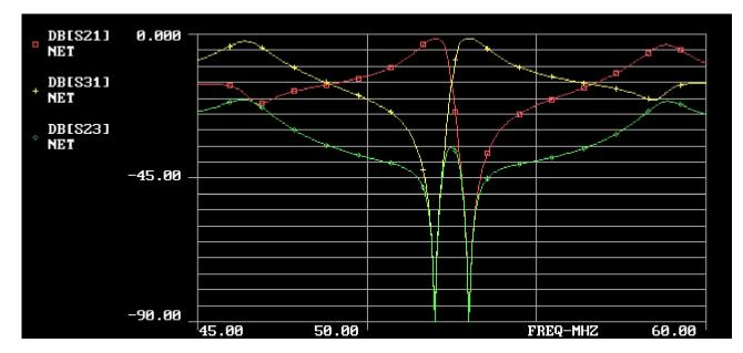
Sweep frequency range 45 MHz to 60 MHz of the 4-stub HR Duplexer encompassing TV CH 2 (54 - 60 MHz). For this sweep the following parameters were measured:
