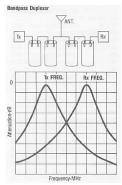
2a) BP - Band Pass, built using tuned/resonant elements which 'pass' one particular frequency in the transmit and receive legs.
