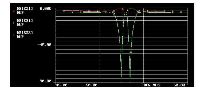
Sweep frequency range 45 MHz to 60 MHz of a 6-stub Notch Duplexer encompassing TV CH 2 (54 - 60 MHz). For this sweep the following parameters were measured:
