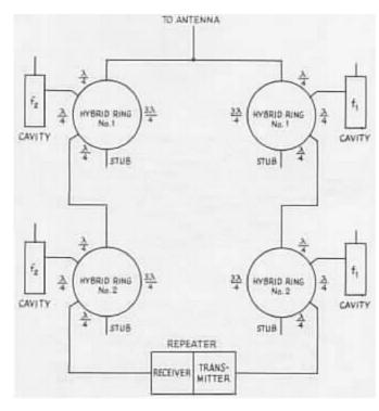
2b) BP - Band Pass, as realized in a Hybrid Ring configuration using tuned/resonant elements which 'notch' one particular frequency in the Hybrid Rings in the transmit and receive legs.
