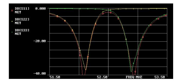
Sweep frequency range 51.5 MHz to 53.5 MHz of the 4-stub HR Duplexer. For this sweep the following parameters were measured:
