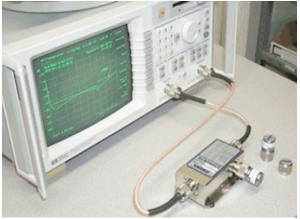
Remove the short from the DUT Port of bridge.
